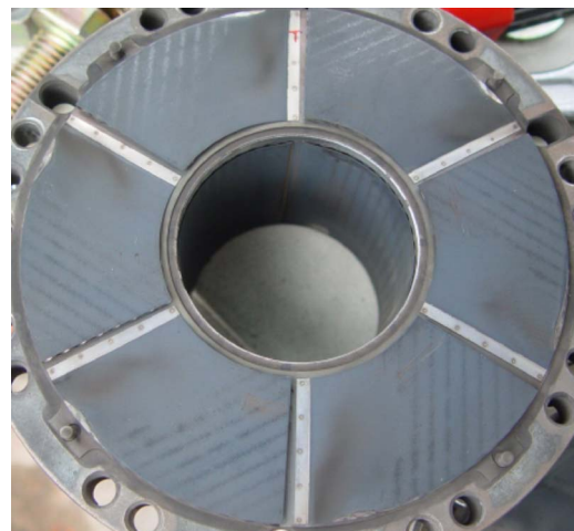
Fig. 16 Bearing wear pattern after a deep surge in the field
